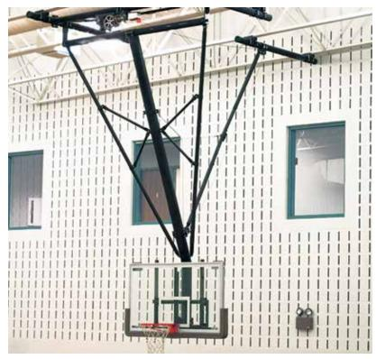
Providing great stability at tall heights, the TB-25S Basketball Backstop's bent stem reduces space between pivot point and jackknife to assist in avoiding obstructions. Backstops are custom designed so the lateral sway brace intersects the main mast at approximately 54" (1.37 m) above the goal and 18" (46 cm) above the backboard; to ensure maximum rigidity.
